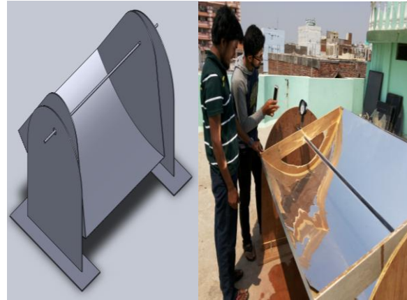
Figure 4: Solid work model and Experimental setup of Solar Parabolic Collector.
