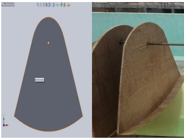
Figure-3: Solid work model and experimental design of Parabolic Ends.
