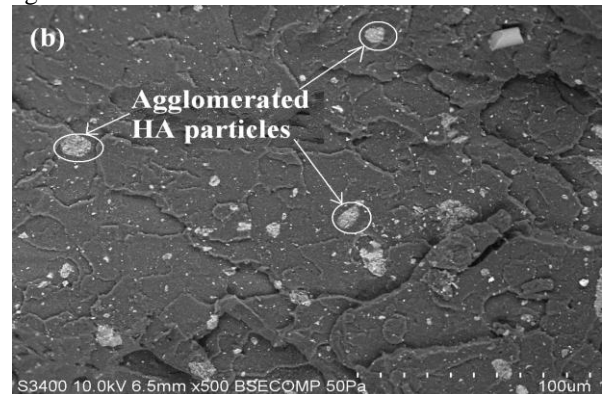
Figure 7. Typical microstructure obtained from the fractured surface of HA/PLA 20 (a) 100X mag. (b) 500X mag.
