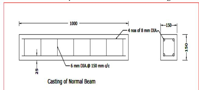
Fig.1 Reinforced Details of Concrete Beam
