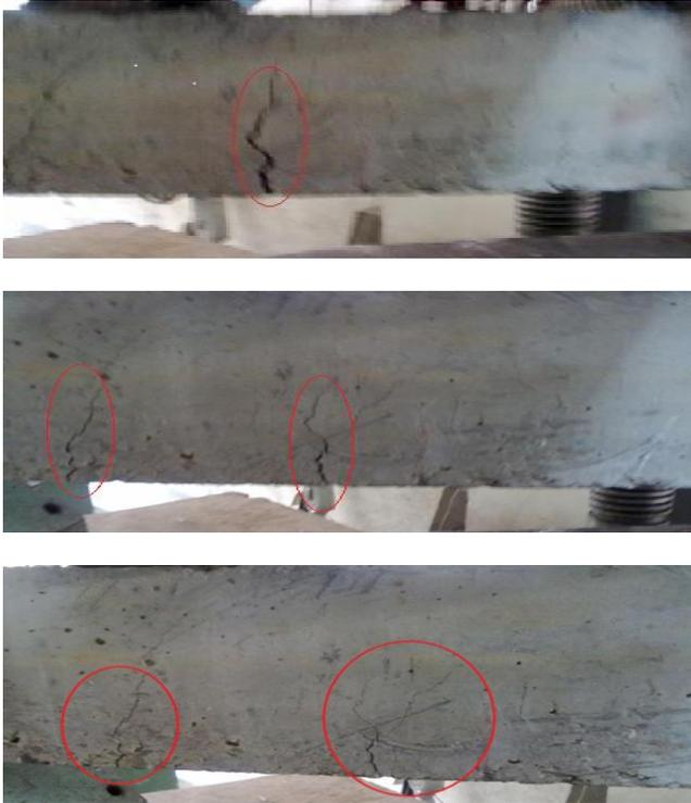
**Fig 9. Cracks in Beams**
