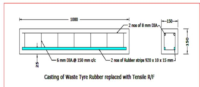
Fig.2 Details of Rubber Reinforced Beam
