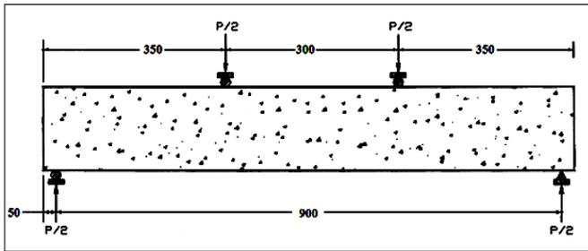
**Fig. 3 Two Point Loading**
