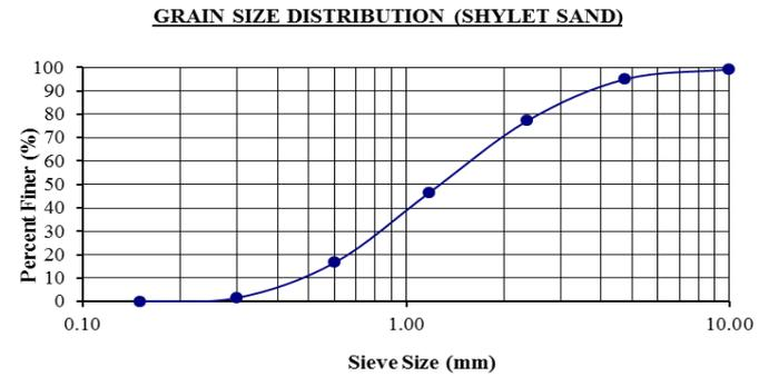
**Figure 2:** Sieve Analysis of Fine Aggregate.
