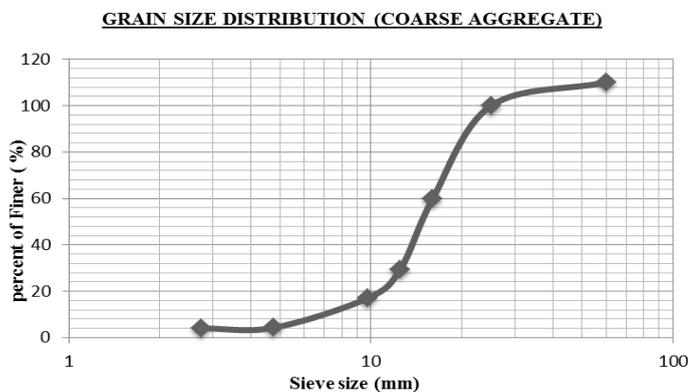
**Figure 1** Sieve Analysis of Coarse
