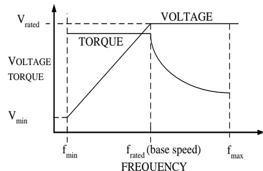
Fig (d) Torque speed characteristics of induction motor with V/f control
