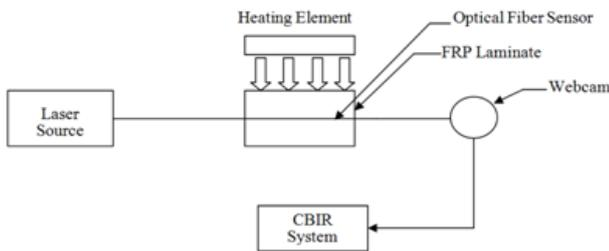
**Figure 2** Schematic illustration of proposed set up
