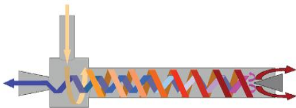
Fig 1: Flow pattern in Vortex tube
