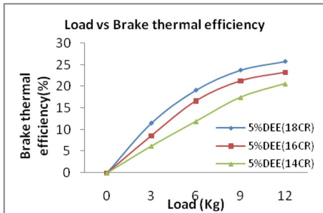
Figure.8. Variation in brake thermal efficiency for 5% DEE blend at different compression ratios
