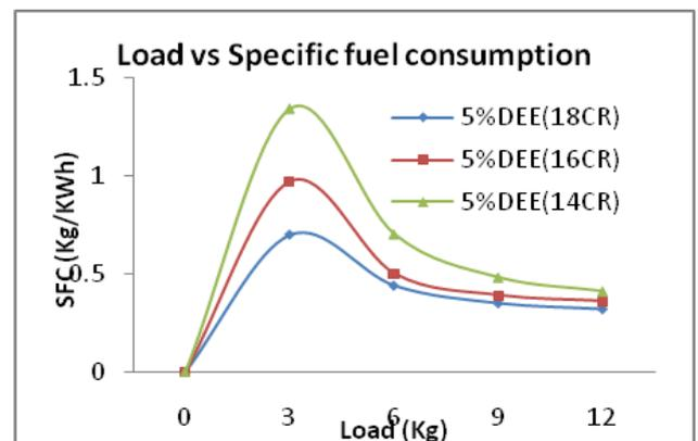
Figure.12. Variation in specific fuel consumption for 5% DEE blend at different compression ratios
