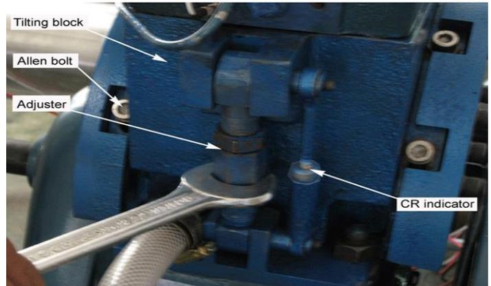
Figure. 2. Compression ratio adjustment
