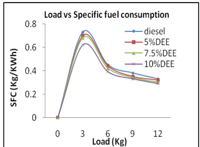
Figure.7 Variation in Specific fuel consumption with load for different blends
