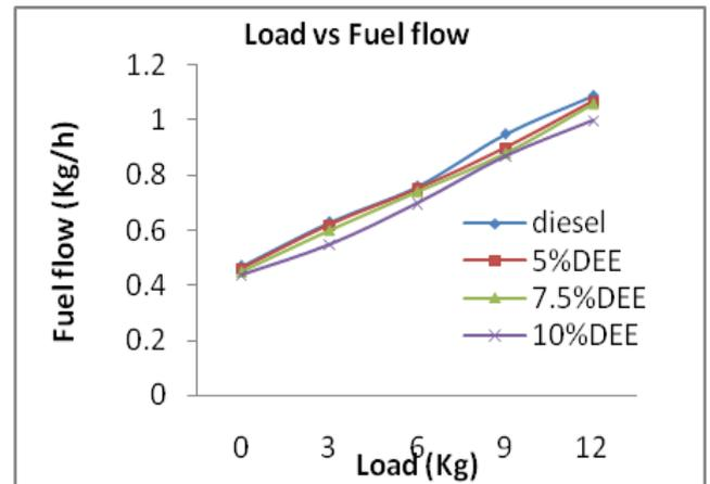
Figure.6 Variation in fuel flow with load for different blends
