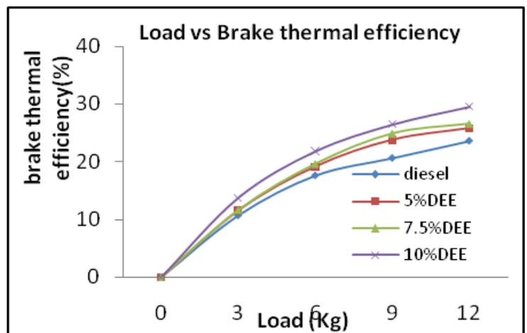
Figure.3. Variation in Brake thermal efficiency with load for different blends
