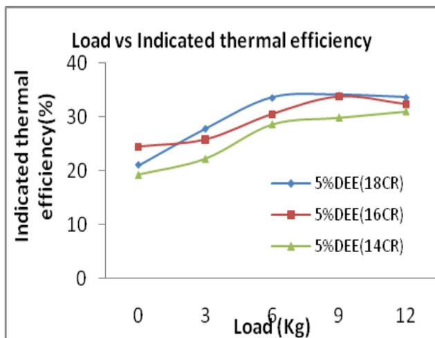
Figure.9. Variation in indicated thermal efficiency for 5% DEE blend at different compression ratios
