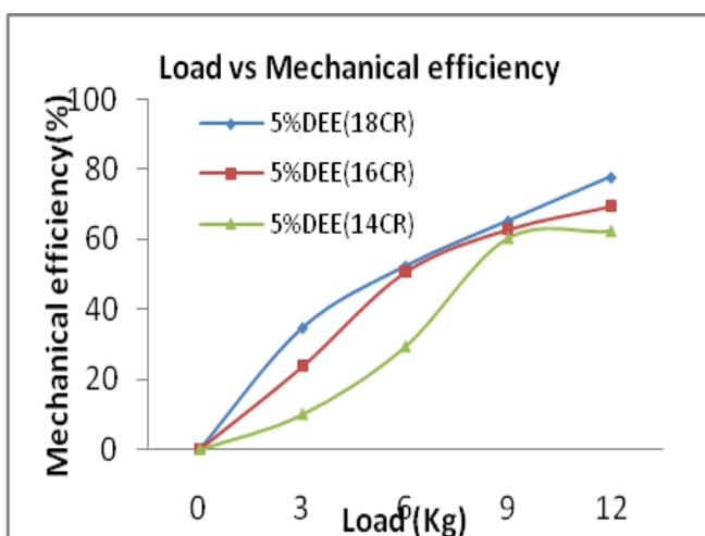
Figure.10. Variation in mechanical efficiency for 5% DEE blend at different compression ratios
