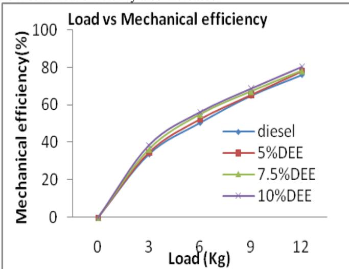
Figure.5 Variation in mechanical efficiency with load for different blends
