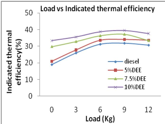
Figure.4 Variation in Indicated thermal efficiency with load for different blends
