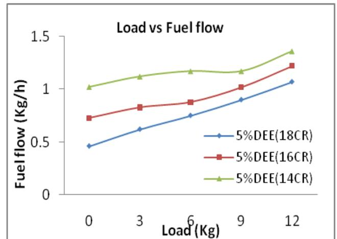
Figure.11. Variation in fuel flow 5% DEE blend at different compression ratios
