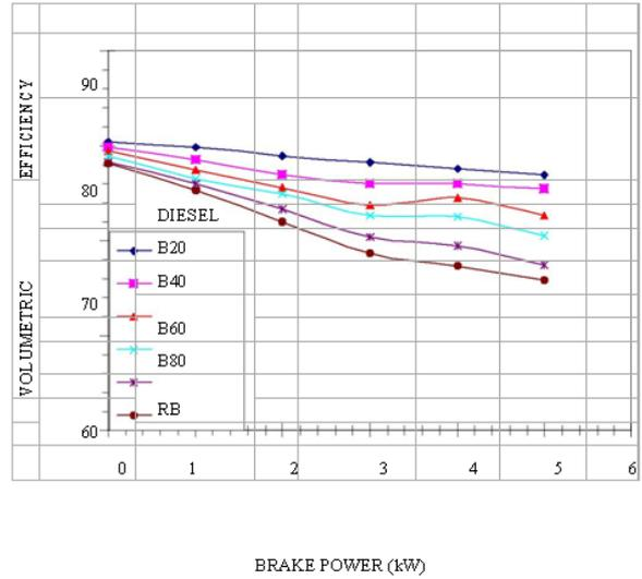
FIGURE 4. VARIATION OF Volumetric Effi. vs. Brake power
