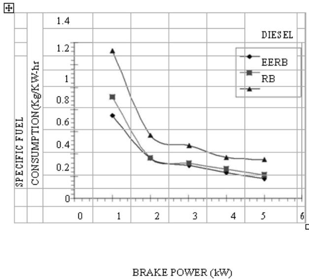
FIGURE 7. VARIATION OF SFC vs. Brake power
