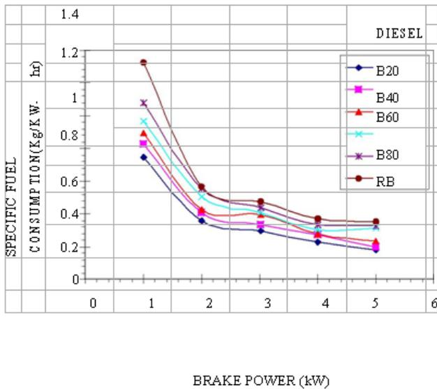
FIGURE 2. VARIATION OF SFC vs. Brake power
