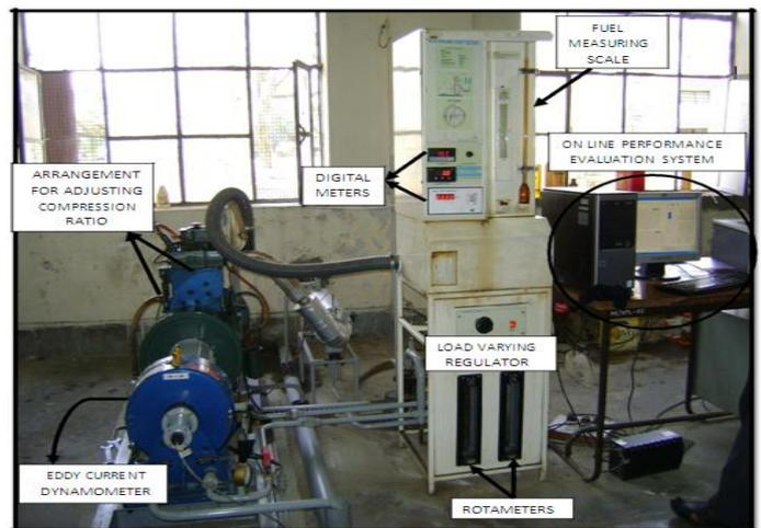
**Figure 1.** Pictorial view of the compression ignition engine.
