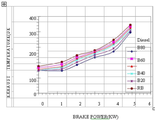
FIGURE 3. VARIATION OF Exhaust temp. vs. Brake power
