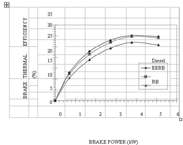
FIGURE 6. VARIATION OF BTE vs. Brake power
