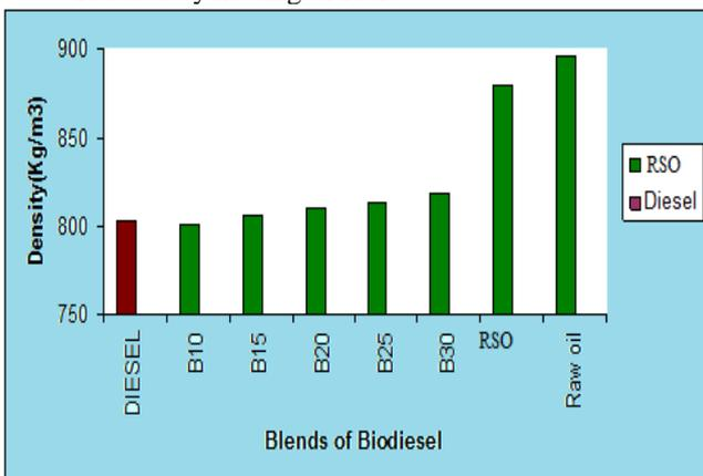
Fig.2: Different Blends of Biodiesel Vs Density
