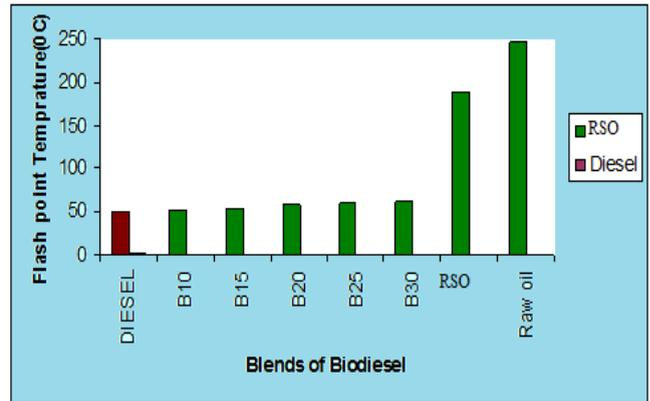
Fig.3: Blends of Biodiesel Vs Flash Point Temperatures
