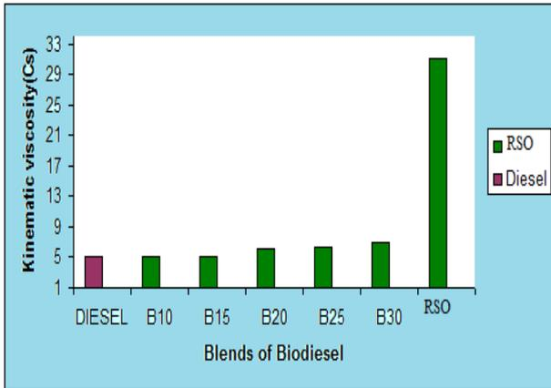
Fig.1: Kinematic Viscosity Vs Blends
