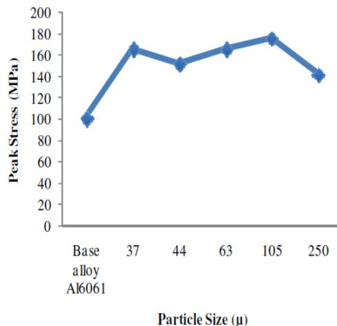
**Figure 6: The Effect of the Particle Size of B<sub>4</sub>C Particulates on the Peak Stress of Stir Cast AMCs**
