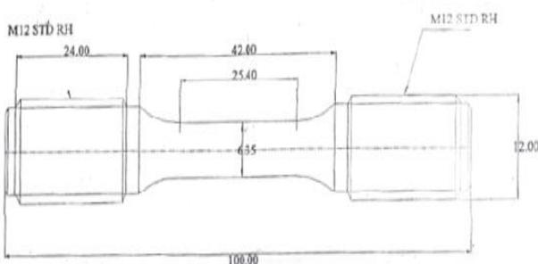
Figure 1: Dimension of Tensile Specimen
