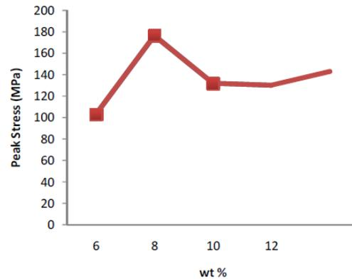
**Figure 7: The Effect of Amount of B<sub>4</sub>C Particulates on the Peak Stress of Stir Cast AMCs**
