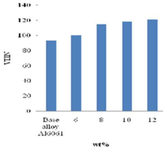
**Figure 5: The Effect of Wt% of B<sub>4</sub>C Particulates on the Hardness of Stir Cast AMCs**
