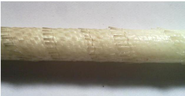
Fig 5 shows fiber glass wrapped shaft
