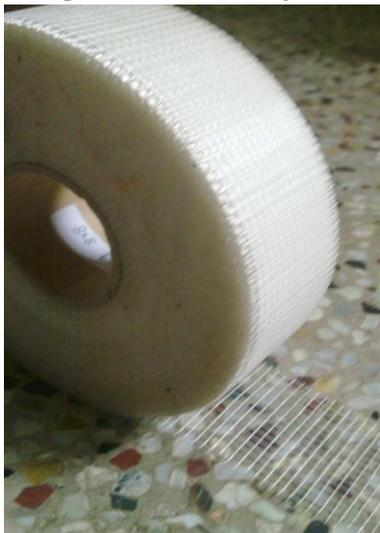
Fig 1 shows fiber glass tape roll
