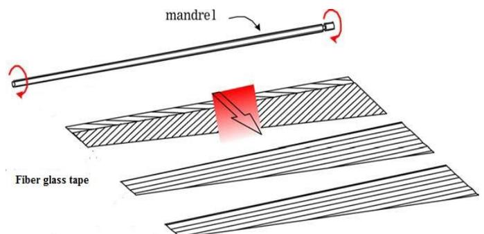
Fig 2 shows application of resin on mandrill
