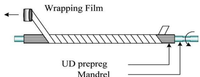
Fig. 3. Wrapping process of the shafts.
