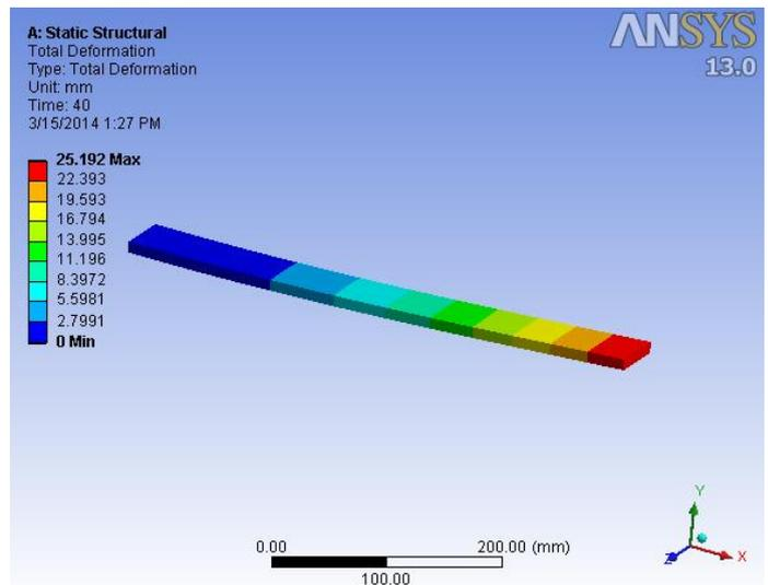
Fig1:Total deformation of Carbon/Epoxy
