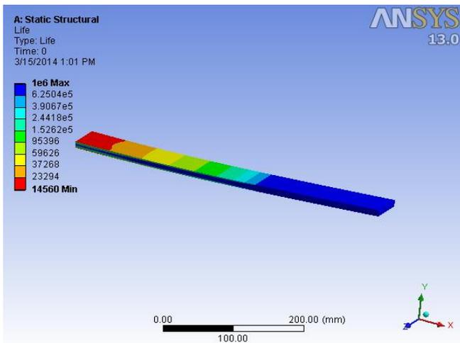
Fig5: Life factor of Carbon/Epoxy
