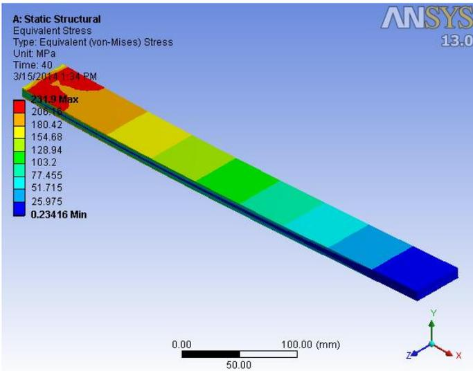
Fig2:Equivalent Stress of steel
