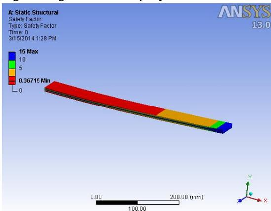
Fig4: Safety factor of Carbon/Epoxy
