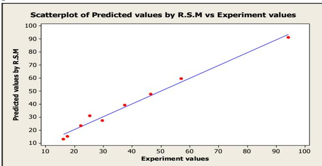
**Fig: 14** Comparison between Experimental values and RSM predicted values of Tensile strength
