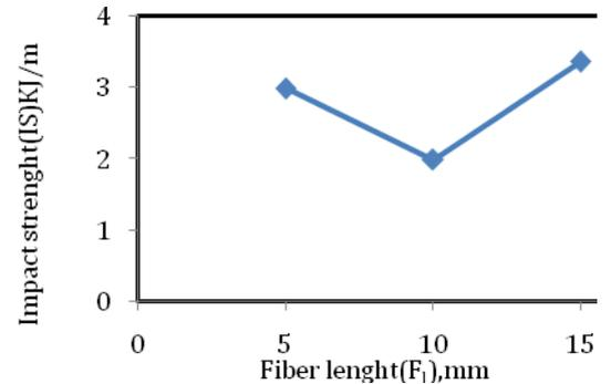
**Fig: 11** Variation of impact strength with respect to fiber length.
