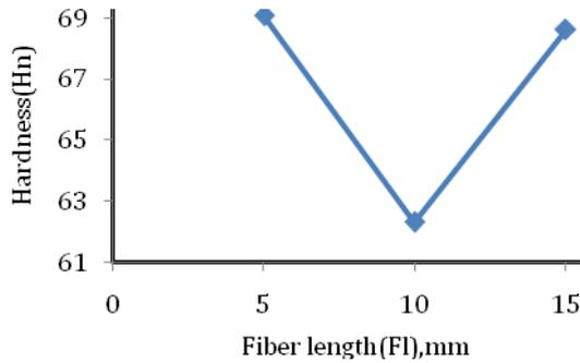
**Fig: 13** Variation of hardness value with respect to fiber length
