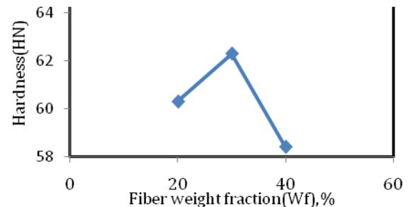
**Fig: 12** Variation of hardness value with respect to fiber weight fraction.
