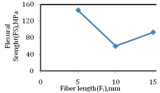
**Fig:9** Variation of flexural strength with respect to fiber length.
