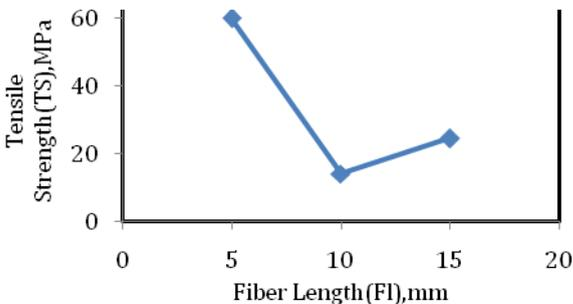
**Fig: 7** Variation of tensile strength with respect to fiber length.
