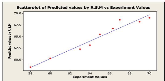
**Fig: 17** Comparison between Experimental values and RSM predicted values of Hardness strength.
