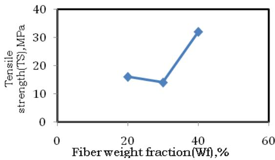
**Fig: 6** Variation of tensile strength with respect to fiber weight fraction.
