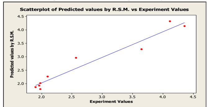
**Fig: 16** Comparison between Experimental values and RSM predicted values of Flexural strength
