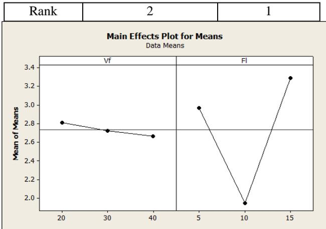
Figure 4 Main effect plots for Impact strength
