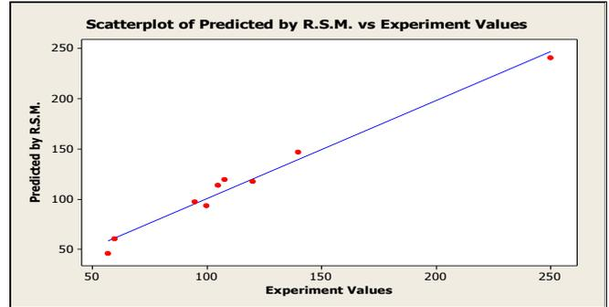
**Fig: 15** Comparison between Experimental values and RSM predicted values of Impact strength
