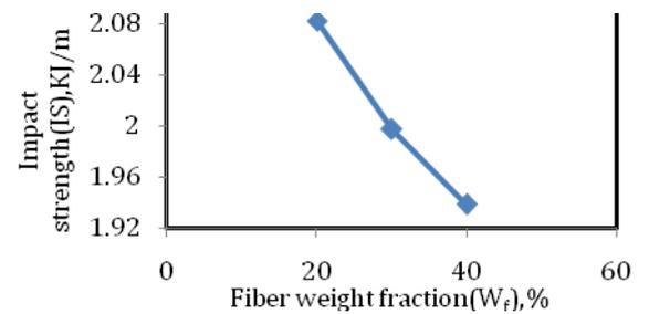
**Fig: 10** Variation of impact strength with respect to fiber weight fraction.
