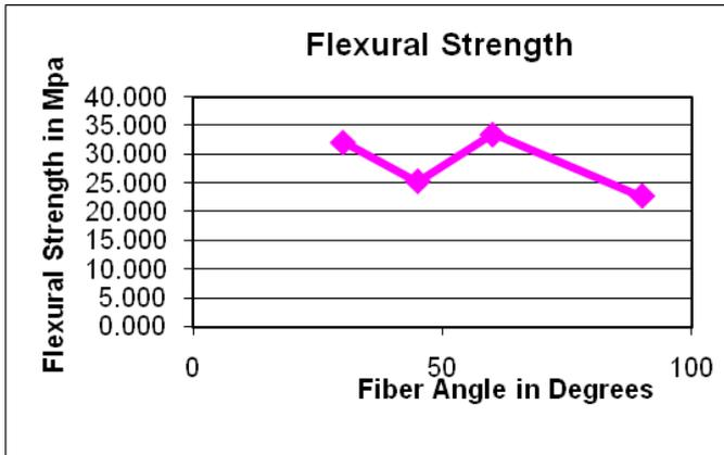
Fig: 5 Flexural strength Vs Fiber angle
