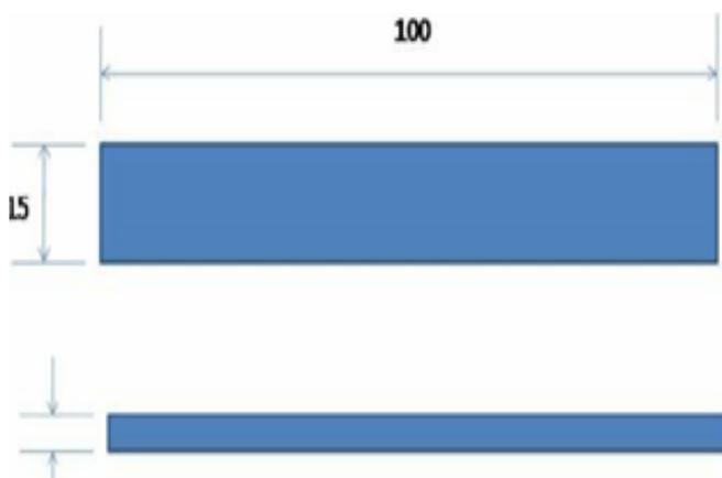
Fig. 2: Specimen for flexural test
