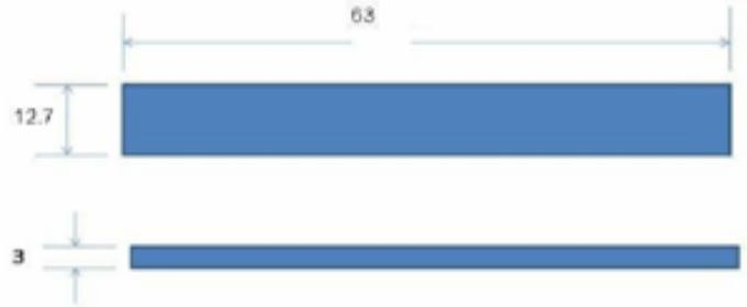
Fig. 3: Specimen for impact test
