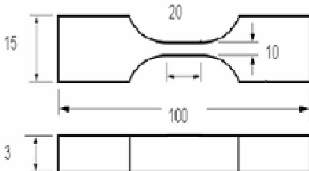
Fig: 1 Dog-bone shaped tensile test specimen (dimensions in mm)
