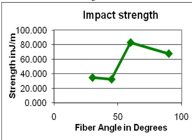
Figure 6 Impact strength Vs Fiber angle
