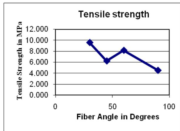
Figure 4 tensile strength Vs Fiber angle
