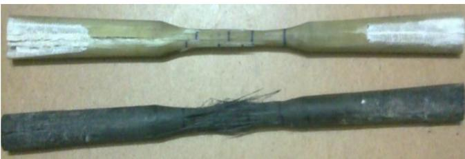
**Figure 7:** Tensile Tested Samples (Glass/Epoxy, Carbon/Epoxy)
