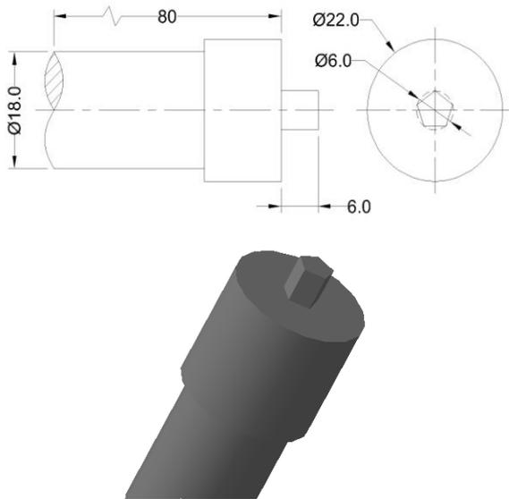
Fig.1 FSW Pentagonal tool
