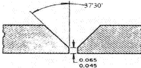
Figure 2 Edge preparations for butt joint.
