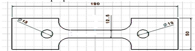
Figure 1 Welding specimen
