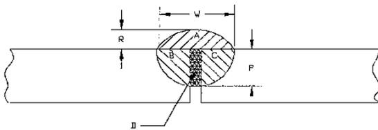
Figure 3 Weld bead geometry.
