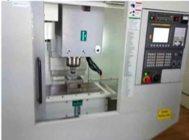
Figure 6: CNC Milling Machine
