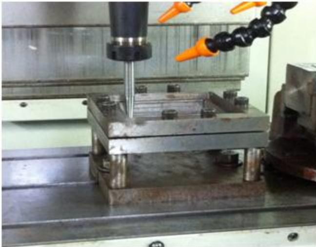
Figure 2 Process of incremental forming
