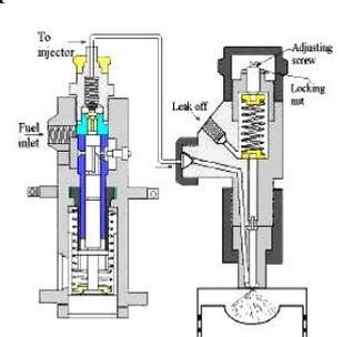
Fig.3 Experimental set up Fig. Bosch fuel pump and fuel Injector
