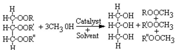
Fig. 2 Process of methyl esterification of rice bran oil. There by obtaining three molecules of methyl ester of the vegetable oil. The chemical reaction is shown in Fig.2. A mixture of anhydrous alcohol and reagent [NaOH] in proper proportions is combined with moisture-free free fatty acid of rice bran oil. The materials are maintained at 40 to 45°C and allowed to settle by gravity for 24 hours.
