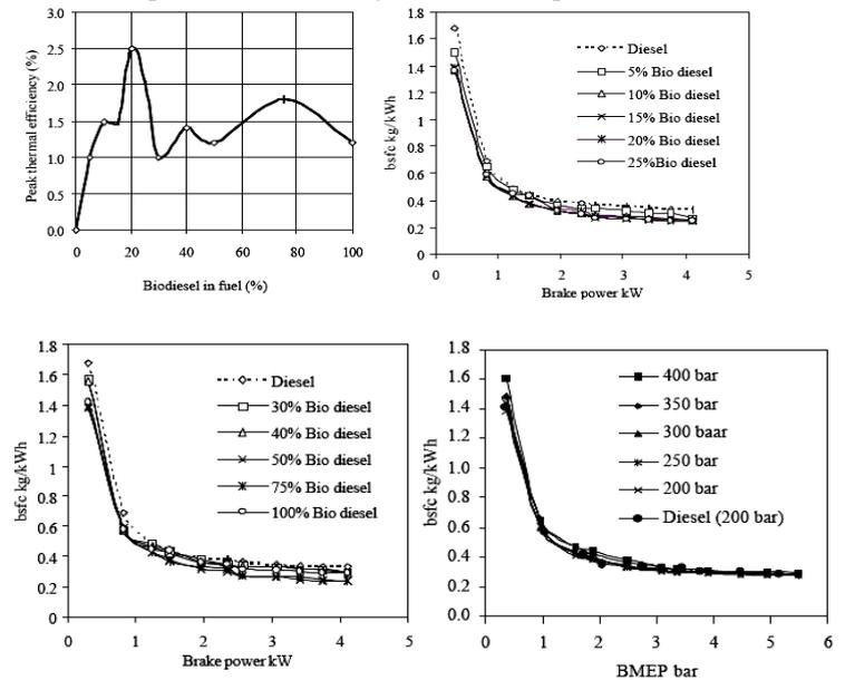
Fig. shows the variation of brake specific fuel consumption at lower concentration of the biodiesel blends. Brake specific fuel consumption of diesel is more when compared with biodiesel blend of 20 percent.
