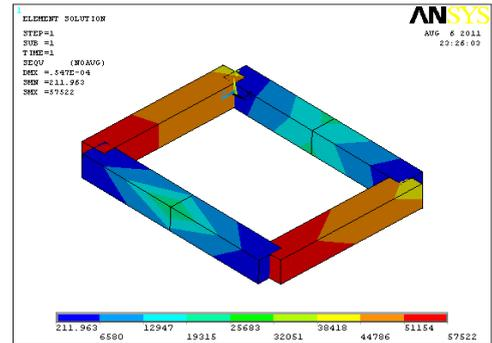
Fig No.5. Maximum stress plot of inner frame
