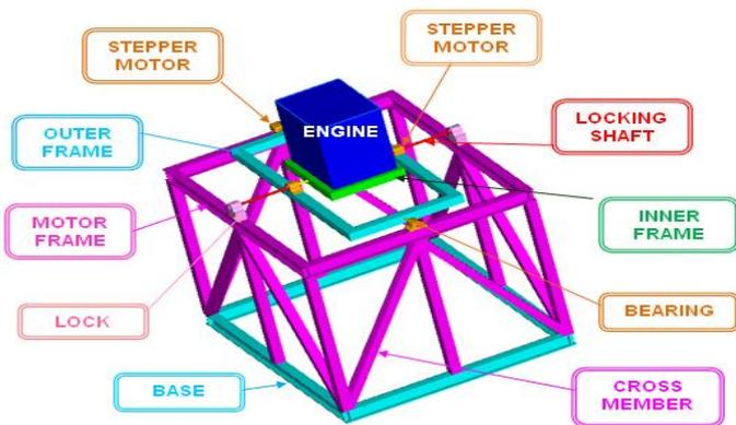
Fig No. 2 Assembly of the intended design of simulator
