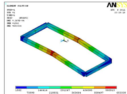
Fig No.6. Maximum stress plot of outer frame
