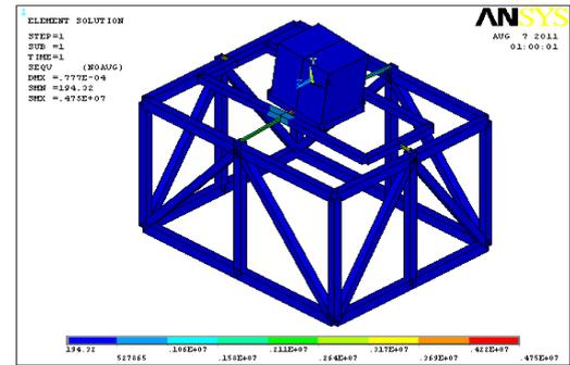
Fig No.4. Maximum stress plot for the entire system
