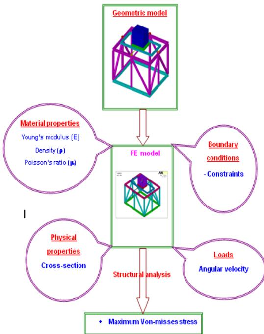
Fig No. 3 Flow Chart of Finite Element Analysis
