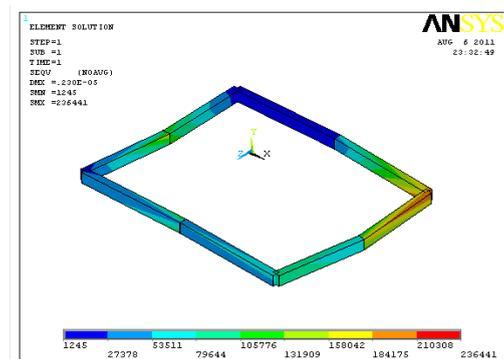
Fig No.7. Maximum stress plot of motor frame
