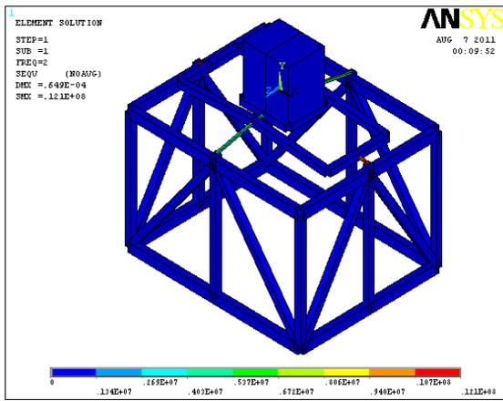
Fig No.9 Dynamic bending stress plot
