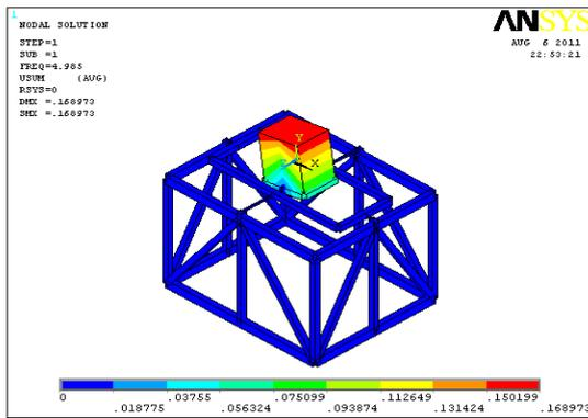
Fig No. 8 First mode shape of the system
