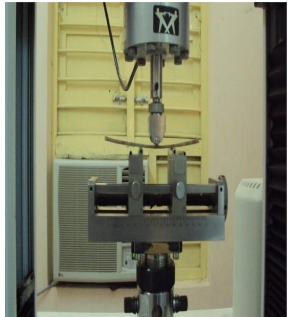
Fig .17. Grip Components for Flexural Test
