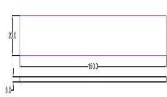
Fig.15. Specimen for Flexural Strength
