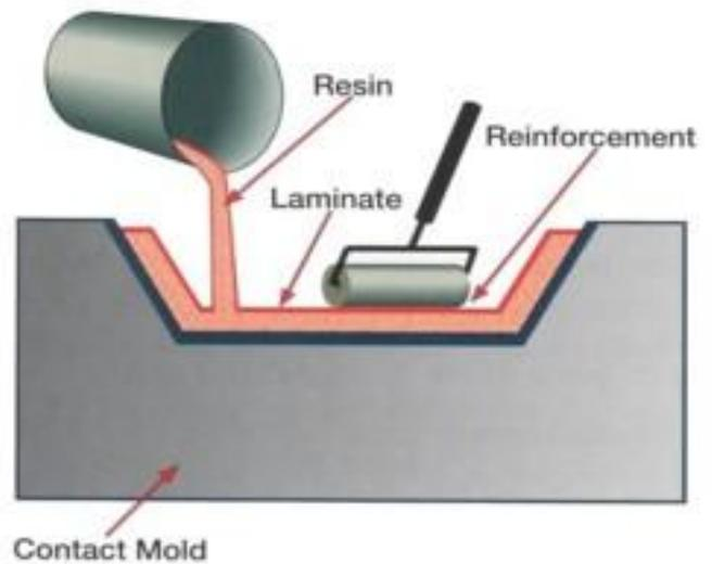
**Fig 4. Hand lay-up technique**
