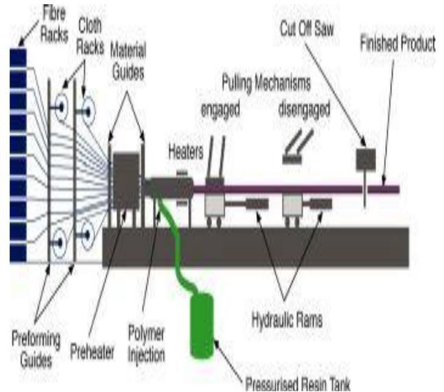
**Fig 8. Pultrusion process**
