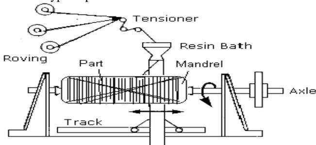
**Fig 7. Filament winding**
