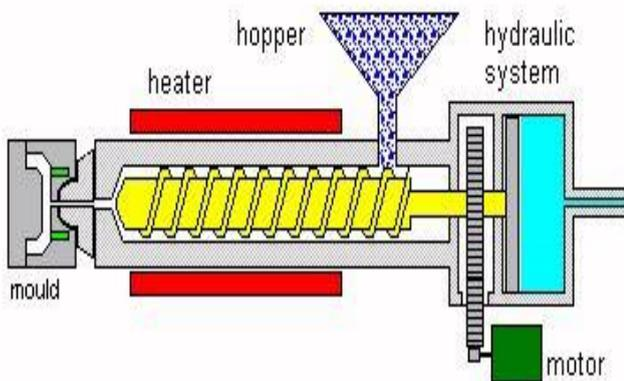
**Fig 6. Injection moulding technique**
