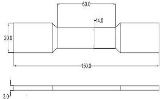
**Fig. 11. Specimen dimensions according to ASTM standards**
