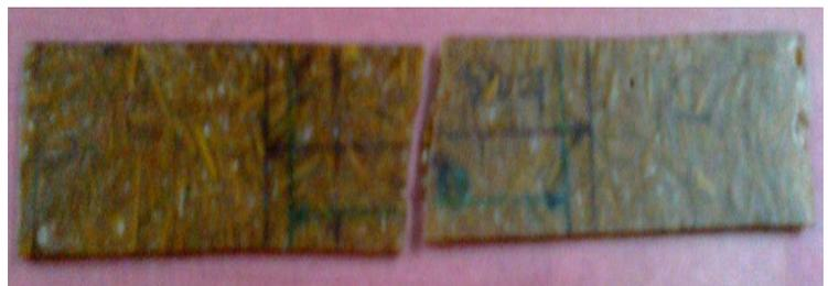
Fig.18. Specimen after Flexural Test
