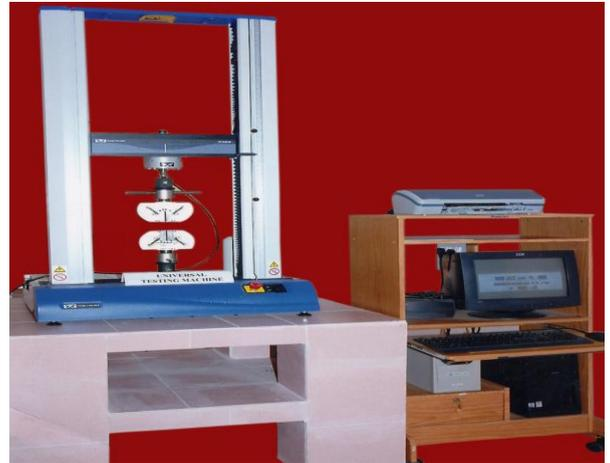
**Fig.10. Universal Testing Machine**
