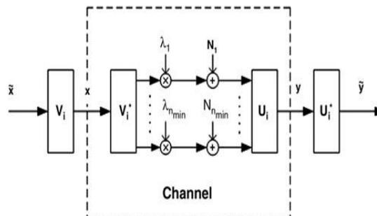
Fig. 2. Converting the MIMO channel into parallel channels by SVD
