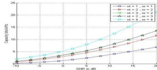
Fig. 3 : Performance analysis of water filling algorithm SNR vs capacity
