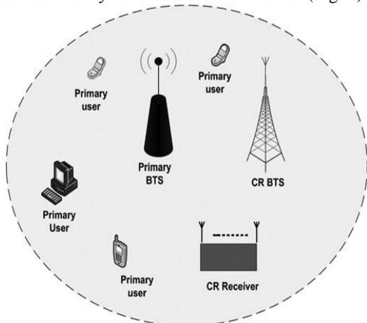
Fig. 1 System design of CR with coexistence of primary and secondary networks .
