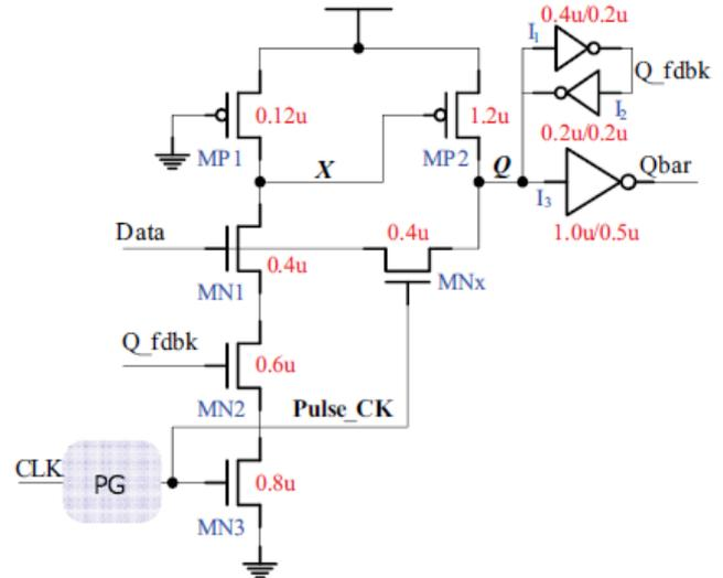
Fig. 2. Schematic of the proposed P-FF design.
