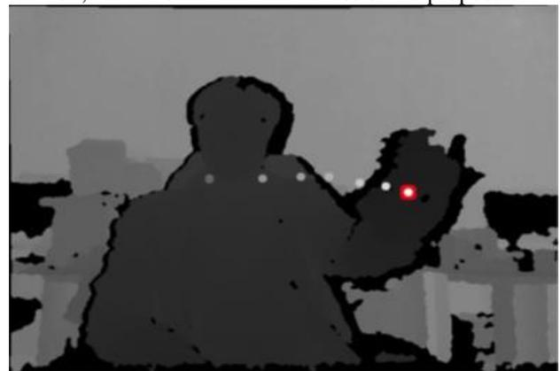
**Figure 6** Hand tracking using kalman filter
