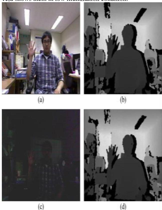
**Figure 1** Comparing color and depth images under different illumination conditions. (a) color image in normal illumination; (b) depth image in normal illumination; (c) color image in low illumination; (d) depth image in low illumination
