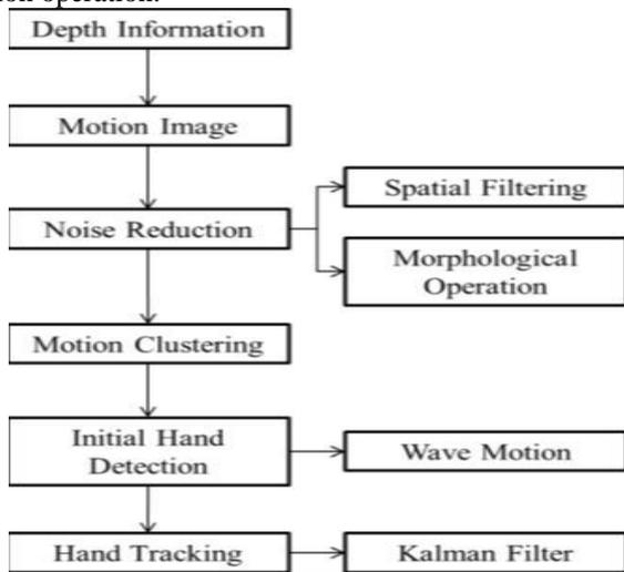
**Figure 3** Procedure of the proposed hand tracking method
