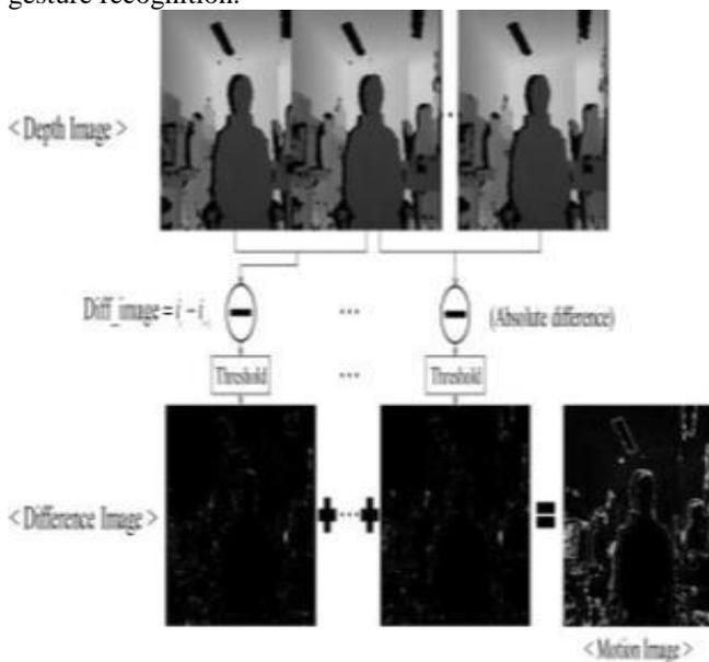
**Figure 4** The process of generating the motion image
