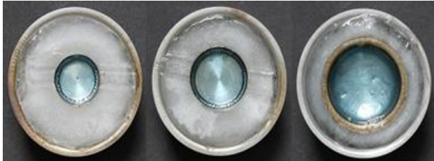
Fig. 2: Bowls filled with ice and fuel; fuel bowls having diameters of 30 mm, 38 mm and 49 mm
