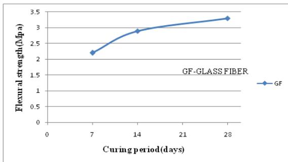
Figure:3.5: Flexural strength with Glass fiber
