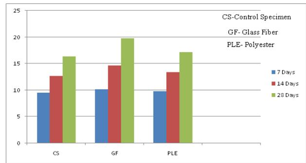
Figure:3.10: Comparison of Compressive strength
