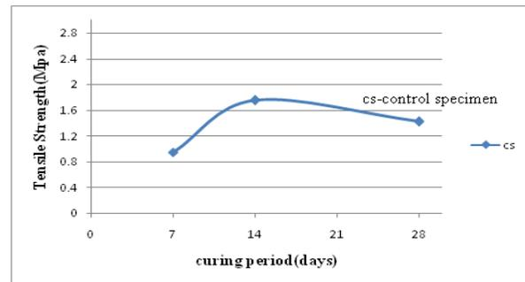
Figure:3.7: Flexural strength without additives
