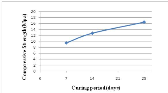
Figure:3.1: compressive strength without additives
