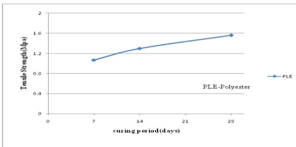
Figure:3.9:Tensile strength with Polyester
