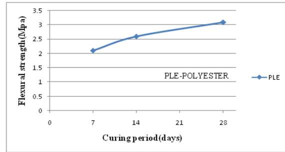
Figure:3.6: Flexural strength with Polyester fiber
