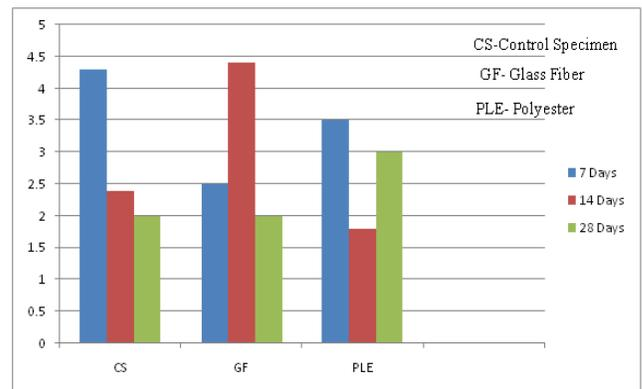
Figure:3.11: Comparison of Flexural strength
