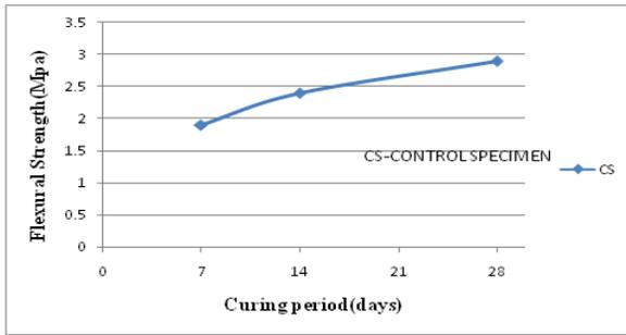
Figure:3.4: Flexural strength without additives
