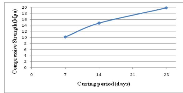
Figure:3.2: compressive strength with Glass fiber
