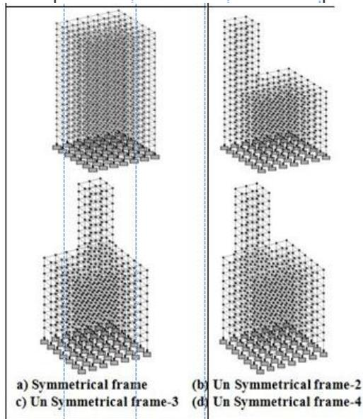
Fig. 2 Selected Frames with Shapes, Supports, Nodes and Framing
