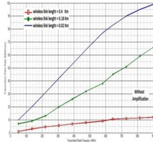
Figure 4 Transmission data rate vs Transmission frequency (without amplification)
