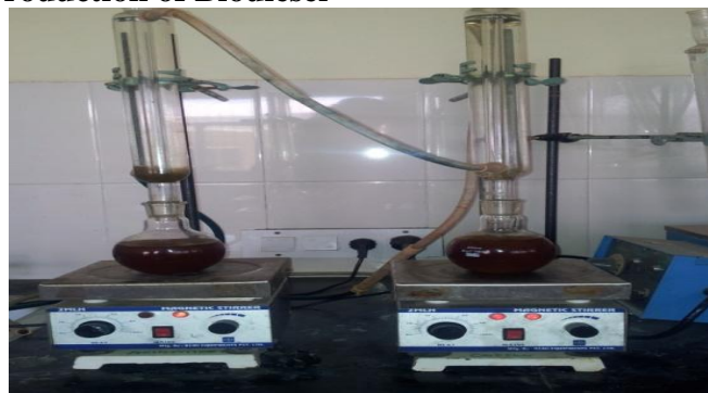
Fig. 1 Setup for production of biodiesel using a magnetic stirrer.
