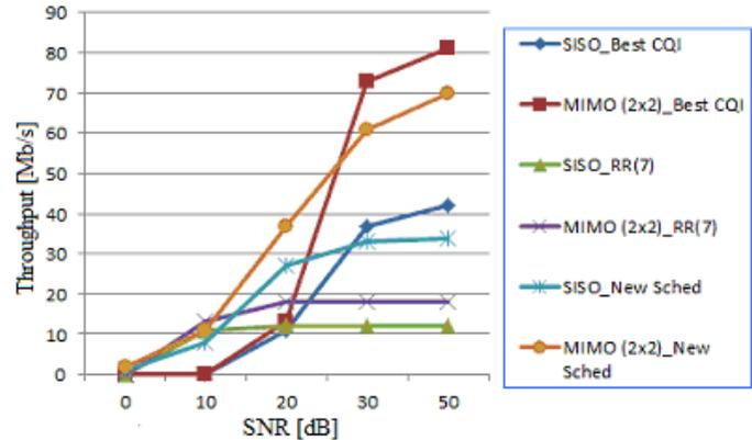
Figure-9: SNR versus Throughput for multiple users (100) comparing different scheduling algorithms.
