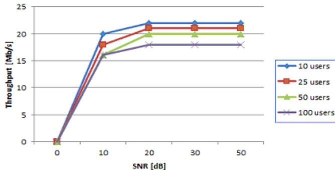
Figure-7: SNR versus Throughput for multiple users in MIMO (2x2) system involving Round Robin algorithm.
