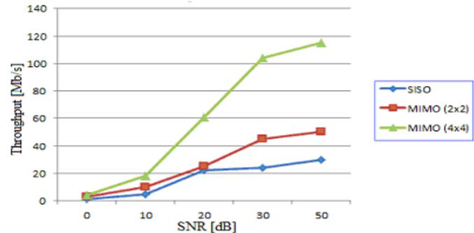
Figure-5: SNR versus Throughput for single user in different transmission schemes involving new scheduling algorithm.
