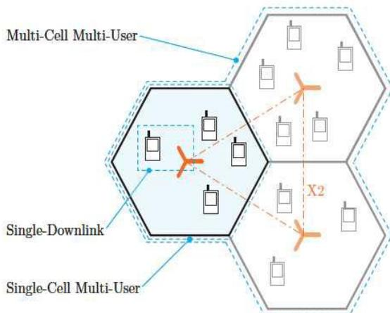
Figure-2: Different simulation scenarios in the LTE simulator.
