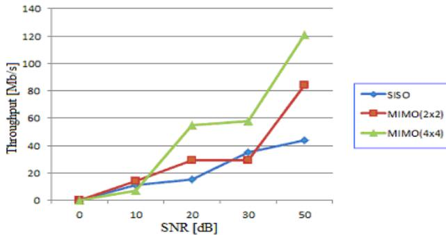
Figure-3: SNR versus Throughput for single user in different transmission schemes involving Best CQI algorithm.
