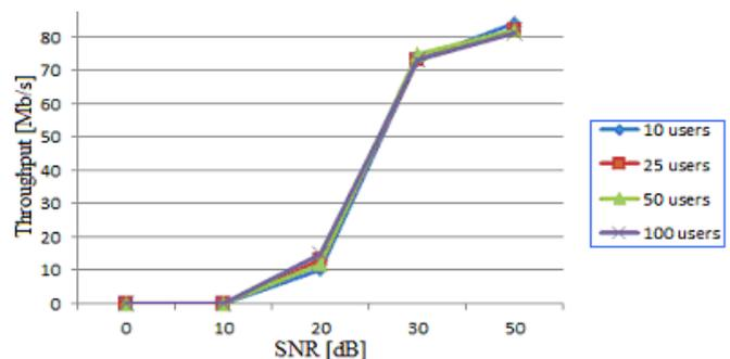
Figure-6: SNR versus Throughput for multiple users in MIMO (2x2) system involving Best CQI algorithm.
