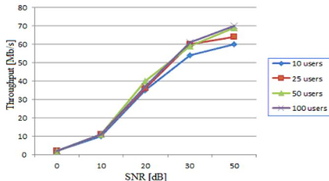
Figure-8: SNR versus Throughput for multiple users in MIMO (2x2) system involving new scheduling algorithm.
