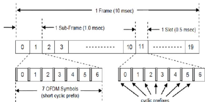
Figure-1: LTE Frame structure
