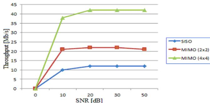
Figure-4: SNR versus Throughput for single user in different transmission schemes involving Round Robin algorithm.
