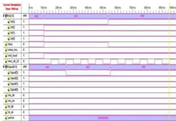
Figure 2 : Simulation Results Of Arbiter Module
