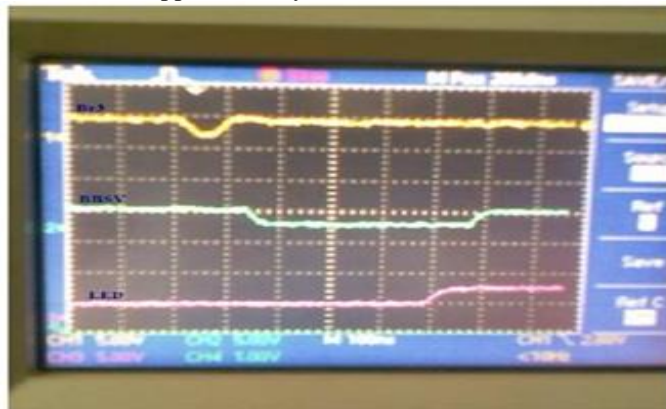
Figure 9: Practical Results when Master resides in slot 2 request for data transfer bus.
