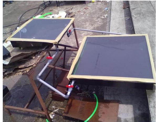
**Solar still combined with the Flat Plate Collector**
