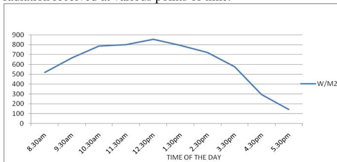
**Radiation vs Time of the Day Day 1 (On Y axis – Radiation intensity W/m<sup>2</sup>)**
