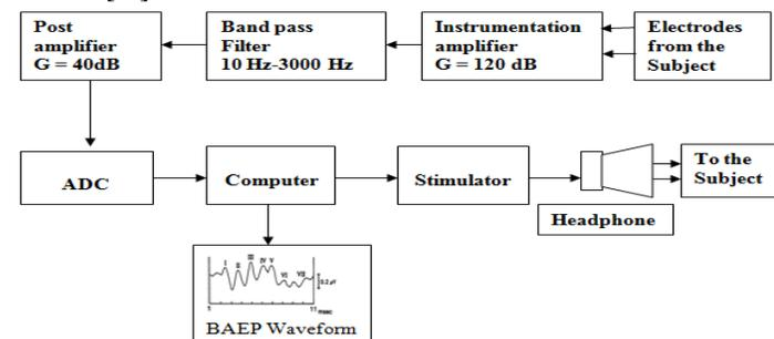
Fig. 1 Recording System of BAEP
