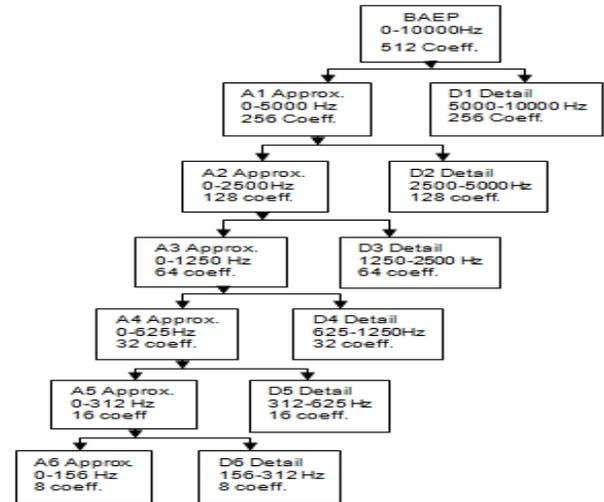
Fig. 4 Decomposition of a BAEP signal for level 6
