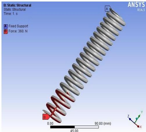
Fig 4: Load applied on Tetra Mesh Mode
