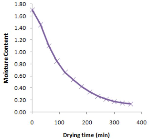
Figure 3.3: Moisture content curve at 60°C
