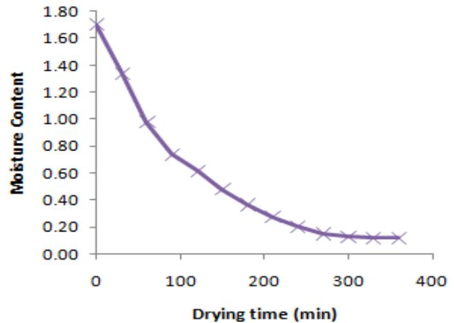
Figure 3.4: Moisture content curve at 70°C
