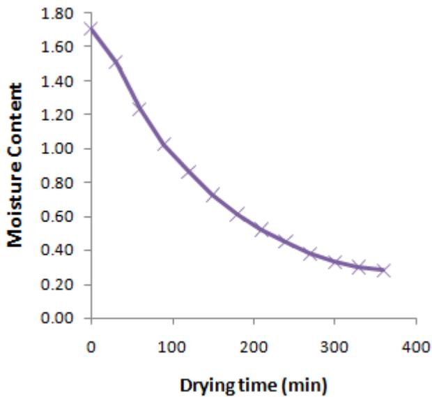
Figure 3.2: Moisture content curve at 50°C
