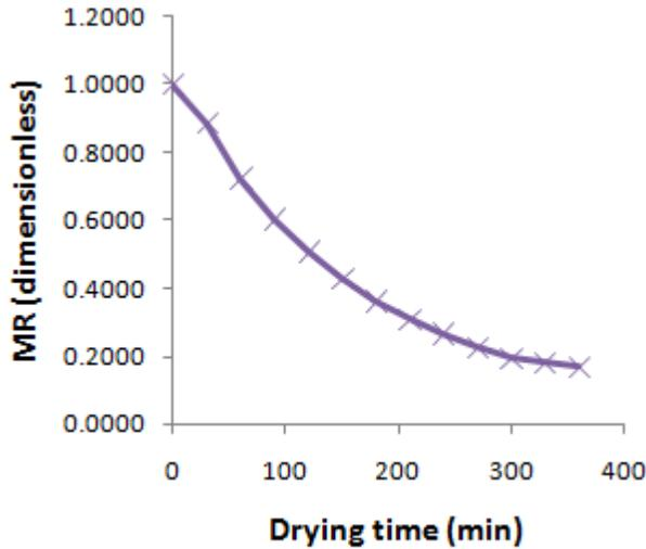
Figure 3.6: Moisture Ratio curve at 50°C
