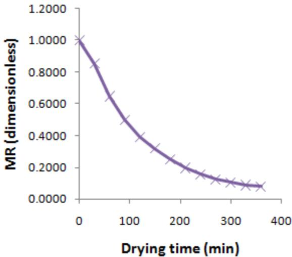
Figure 3.7: Moisture Ratio curve at 60°C
