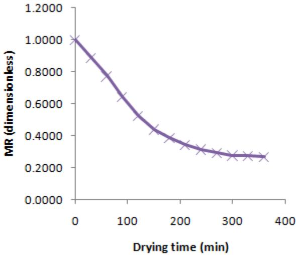
Figure 3.5: Moisture Ratio curve at 40°C
