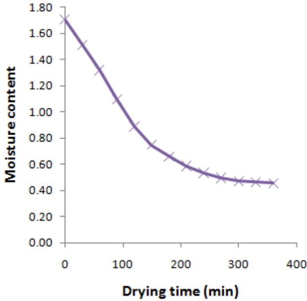
Figure 3.1: Moisture content curve at 40°C
