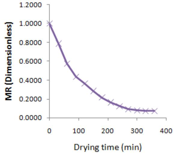
Figure 3.8: Moisture Ratio curve at 70°C
