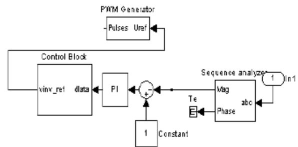
Figure:2 Block diagram of Controller System
