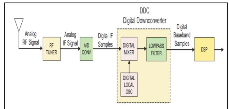
Figure 2-SDR Receiver block diagram
