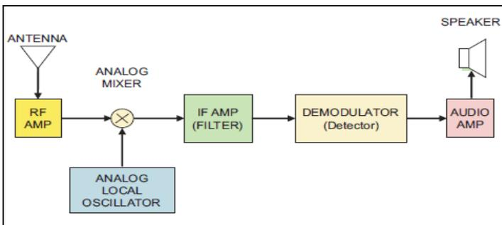
Figure 1-Analog Radio Receiver Block Diagram
