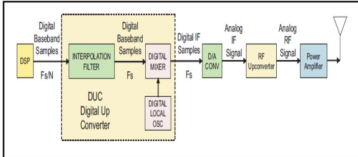
Figure 3-SDR Transmitter Block Diagram
