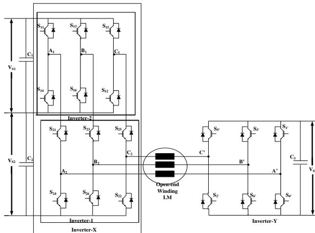
Fig.2 schematic of inverter fed open end winding I.M drive
