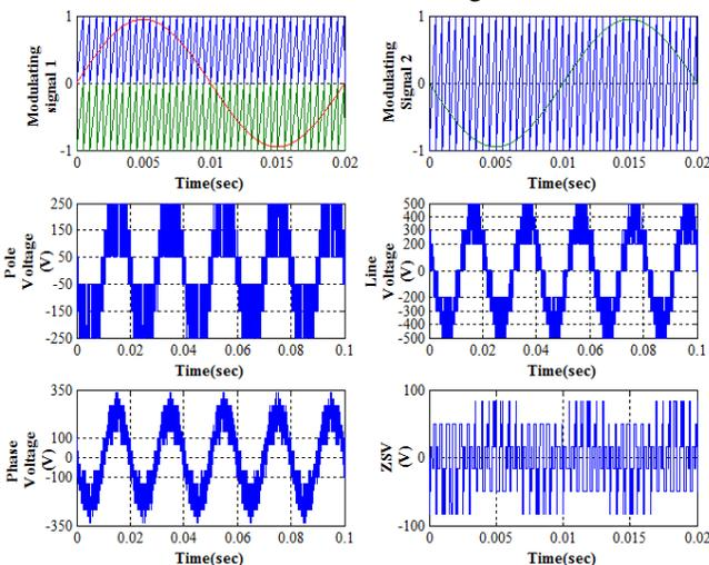
Fig.4 Modulating signal, Pole voltage, Line voltage, phase voltage, ZSV for 6-level inverter using SPWM
