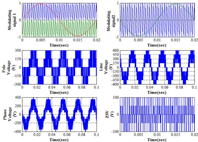
Fig.3 Modulating signal, Pole voltage, Line voltage, phase voltage, ZSV for 5-level inverter using SPWM
