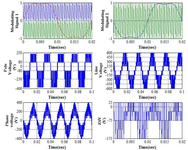
Fig.9 Modulating signal, Pole voltage, Line voltage, phase voltage, ZSV for 5-level inverter using THIPWM
