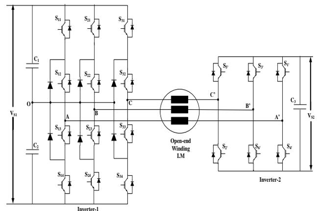
Fig.1 Schematic of proposed inverter fed open end winding I.M drive
