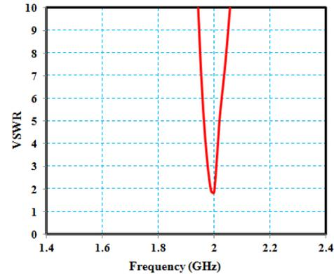
Fig. 8. VSWR plot of the suggested Steerable antenna.
