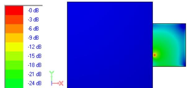
Fig. 5. Surface current distribution of the suggested antenna at 2 GHz.
