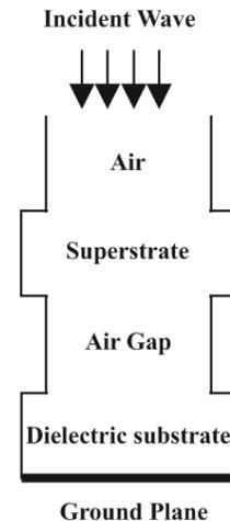
Fig. 2. Equivalent Transmission line model of the suggested antenna structure (figure 1a).
