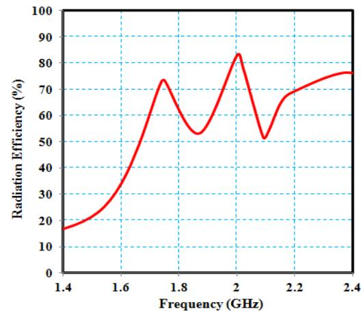
Fig. 9. Radiation Efficiency of the suggested Steerable Antenna.
