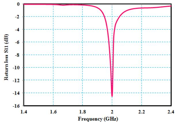
Fig. 4. Return loss characteristic  $|S_{11}|$  of the suggested steerable Antenna.
