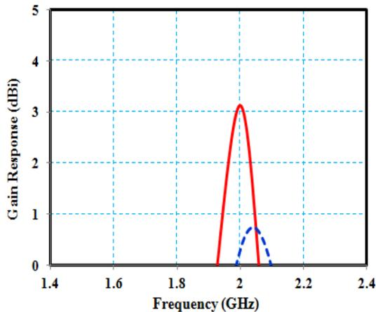
Fig. 10. Gain of the suggested steerable antenna.
