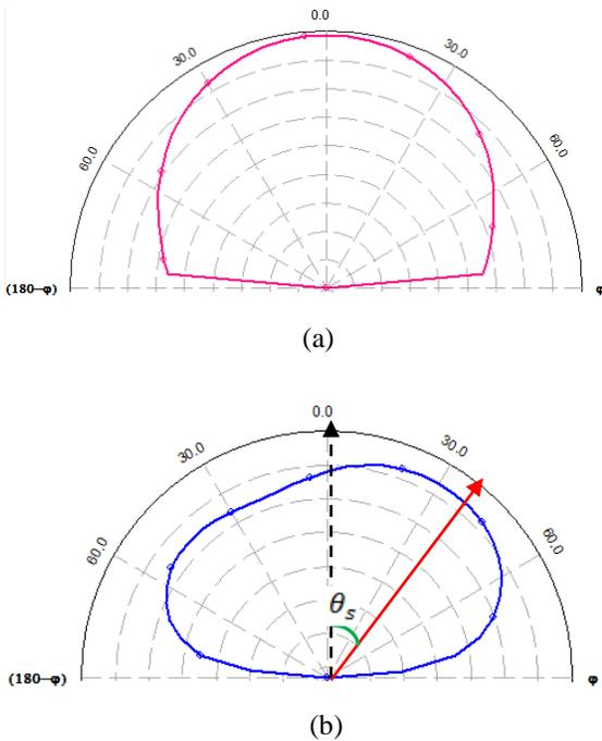
Fig. 6. Simulated 2D Radiation pattern of the suggested steerable antenna.
