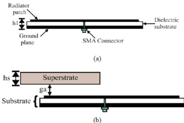
Fig. 1. Cross sectional view of the suggested antenna.
