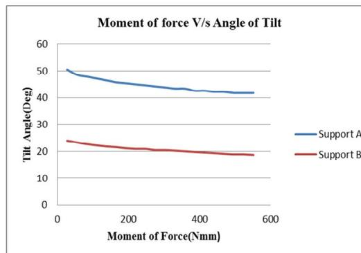
Figure no. 6: Moment of force V/s Tilt angle Case 2 ( $L/4$ ;  $A=75$ ,  $B=225$ )
