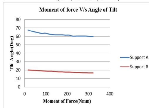
Figure no. 8: Moment of force V/s Tilt angle Case 4( $L/4$ ;  $A=37.5$ mm,  $B=262.5$ mm)
