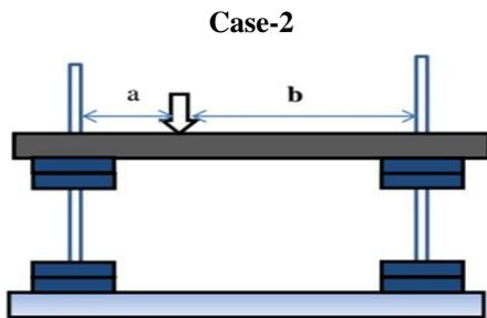
Figure no. 2: Eccentrically located Point load
