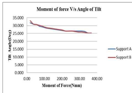
Figure no. 5: Moment of force V/s Tilt angle Case 1( $L/2$ ;  $A=B=150$ mm)
