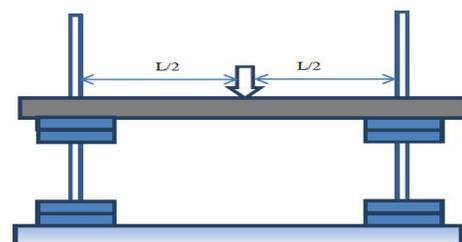
**Figure no. 1: Centrally located Point load**
