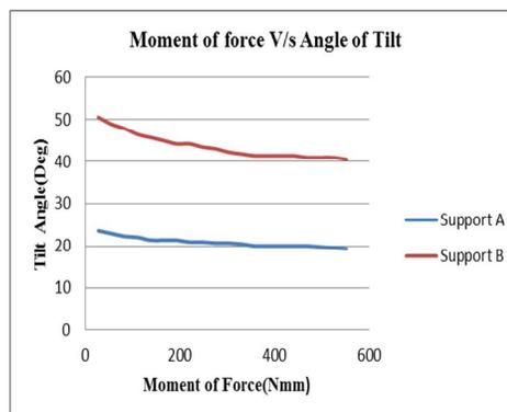
Figure no. 7: Moment of force V/s Tilt angle Case 3( $L/4$ ;  $A=225$ ,  $B=75$ )
