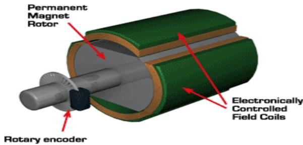
Figure 6: Outer structure of BLDC motor
