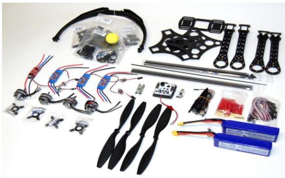
Figure 3: Different parts of Quad copter
