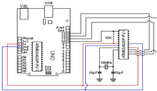
Figure 17 Block diagram of Microcontroller
