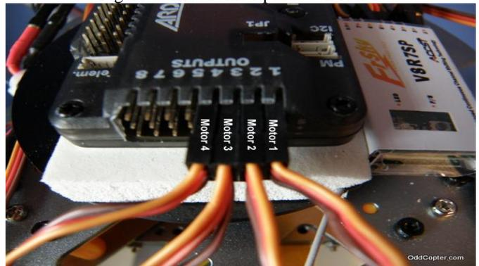
Figure 9: Motor outputs from the APM to the Motors through the ESC
