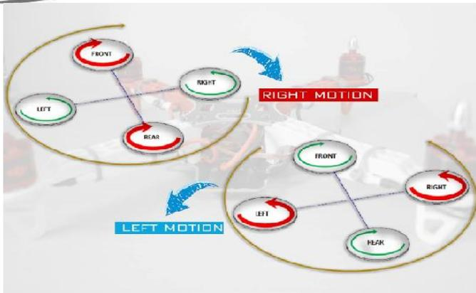
Figure 15: Left and Right motion
