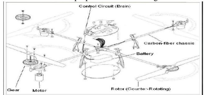
Figure 4: Structure of Quad copter
