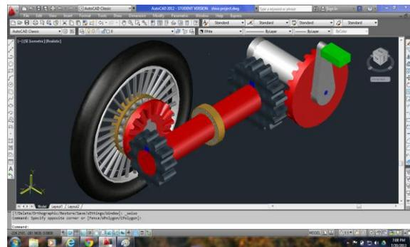
Fig:6.Final gears arrangement
