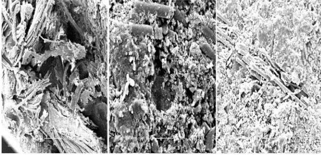
**Fig. 5.2: Untreated Aegle Marmelos fiber 200X magnification (Straight, Slant and Criss-cross orientations)**
