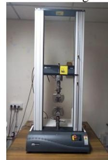
**Fig. 4.1: UTM for tensile and flexural tests**
