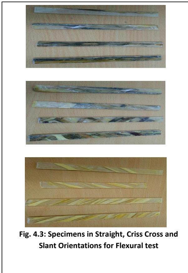
**Fig. 4.3: Specimens in Straight, Criss Cross and Slant Orientations for Flexural test**
