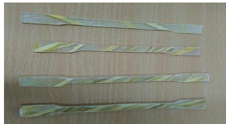
**Fig. 4.2: Specimens in Straight, Criss Cross and Slant Orientations for tensile test**
