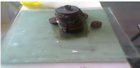
**Figure 1.** Mould covered with Glass plate with weights on it
