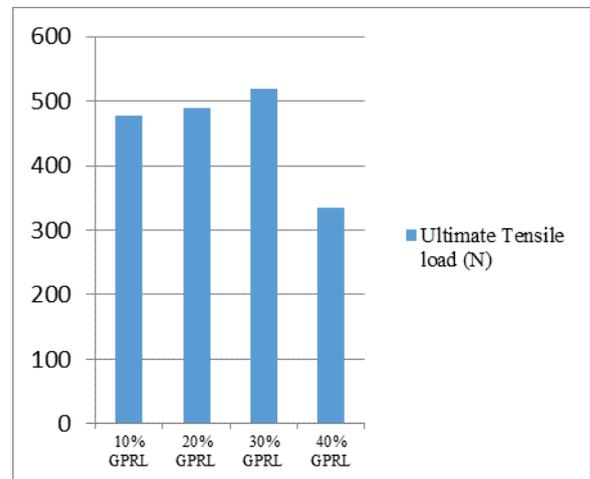
**Figure:8** Ultimate Tensile Load vs GPRL's
