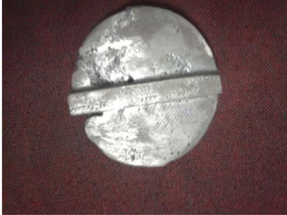
Figure 1. Casting made using investment casting rapid prototyping approach
