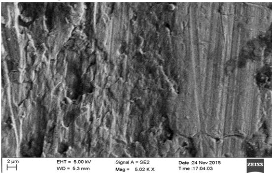
Fig 11: SEM micrograph (SE mode) for flood coolant machining
