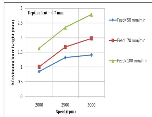
**Fig.9: Variation of maximum burr height with spindle speed at different feed rates in flood coolant machining**
