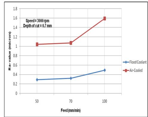
**Fig.3: Variation of surface roughness with feed rate in flood coolant and air-cooled machining for expt. 3**
