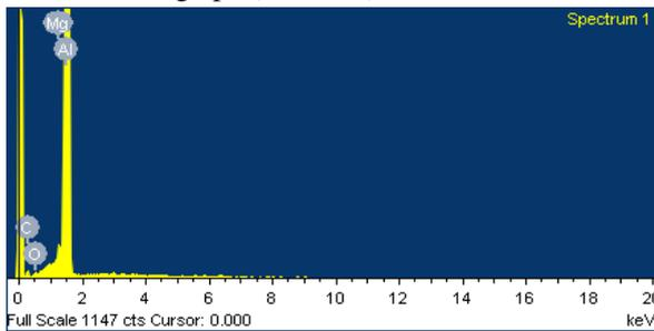
Fig 12: EDS pattern for the surface after flood coolant machining
