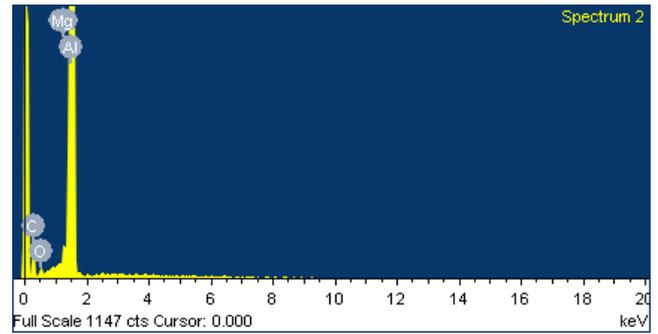
Fig 14: EDS pattern for the surface after air-cooled machining
