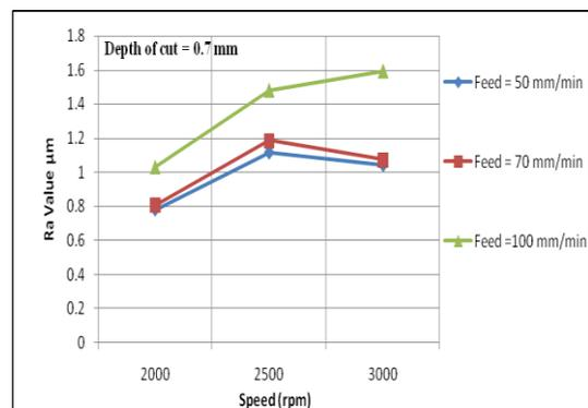
**Fig.5: Variation of surface roughness with speed at different feed rates in air cooled machining**
