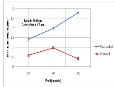
**Fig.8 Variation of maximum burr height with feed rate in flood coolant and air-cooled machining for expt. 3**
