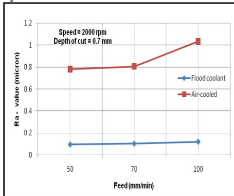
**Fig.1: Variation of surface roughness with feed rate in flood coolant and air-cooled machining for expt. 1**
