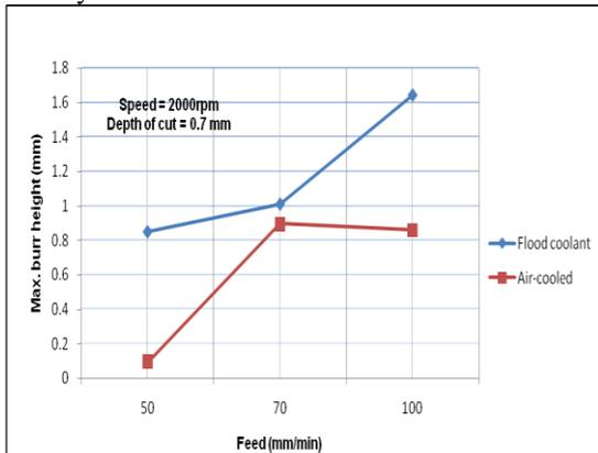
**Fig.6 Variation of maximum burr height with feed rate in flood coolant and air-cooled machining for expt. 1**
