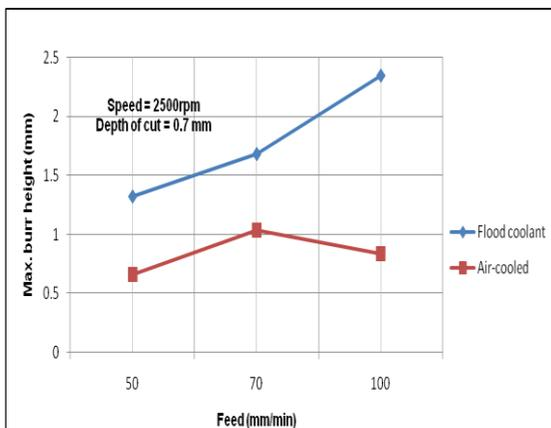
**Fig.7 Variation of maximum burr height with feed rate in flood coolant and air-cooled machining for expt. 2**
