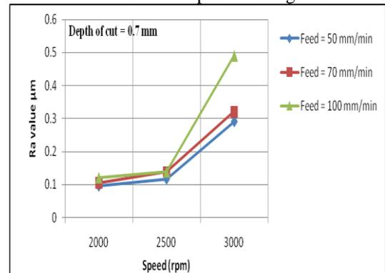
**Fig.4: Variation of surface roughness with speed at different feed rates in flood coolant machining**
