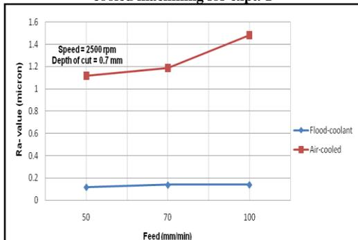
**Fig.2: Variation of surface roughness with feed rate in flood coolant and air-cooled machining for expt. 2**
