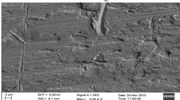
Fig 13: SEM micrograph (SE mode) for air-cooled machining
