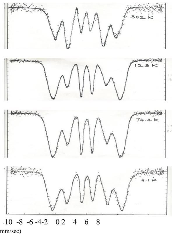
Figure 2: Mossbauer Spectra of amorphous  $Fe_{76}Pr_4B_{20}$  alloy at different temperatures.
