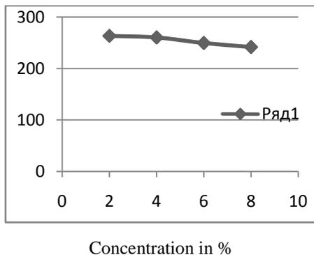
Figure 6 Concentration dependence of the effective magnetic field ( $H_{\text{eff}}$ ) of amorphous  $\text{Fe}_{80-x}\text{Pr}_x\text{B}_{20}$  ( $2 \leq X \leq 8$ ) alloy for  $X = 2\%$ ,  $4\%$ ,  $6\%$  &  $8\%$
