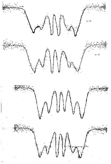
Figure 5 Mossbauer Spectra of Amorphous  $\text{Fe}_{80-x}\text{Pr}_x\text{B}_{20}$  ( $0 \leq X \leq 8$ ) alloys at 4.2 K for  $X = 2\%$ ,  $4\%$ ,  $6\%$  and  $8\%$  (from bottom)
