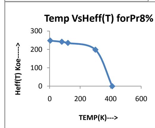
Figure 3: Temperature dependence of effective magnetic hyperfine field  $H_{eff}(T)$  of amorphous  $Fe_{80-x}Pr_xB_{20}$  ( $x=2,4,6,8$ ) alloy
