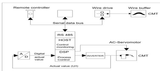
Fig. 1: Fronius CMT-GMAW process control diagram [ i ]
