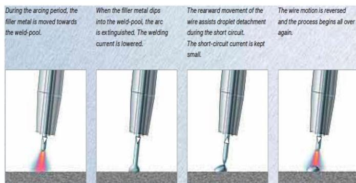
Fig. 3: CMT-GMAW wire retraction process[i]
