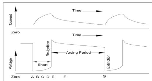
Fig. 2: Schematic representation of short circuiting metal transfer.
