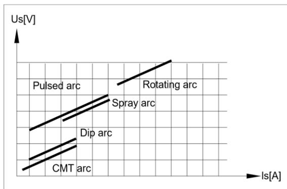
Fig. 4: Comparative thermal inputs for various metal transfer processes.
