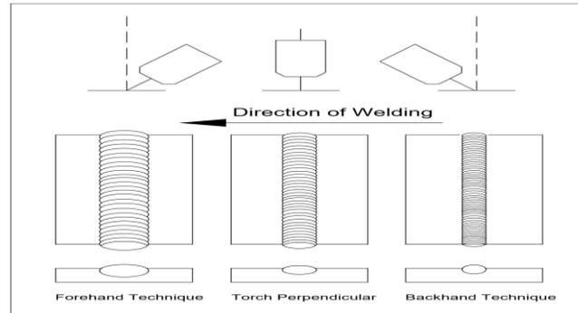
Fig. 5: Effect of electrode position and welding technique
