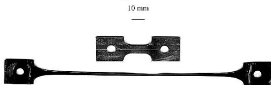
Superplasticity, as referred to in this paper, is described as the capability of a material to undergo extensive tensile
