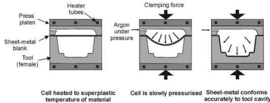
Various pressures were applied and parameter like deformation with respect to time, thickness variations of cup and micro structure were studied.
