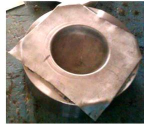
Fig 3.3 super plastically Formed material
